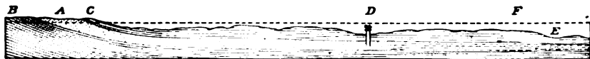
FIG. 3.—Section showing transition from porous to impervious bed. As the bed A is inclosed between impervious beds B and C , an artesian well is obtained at D . At E , however, A is impervious and water can not be obtained.
